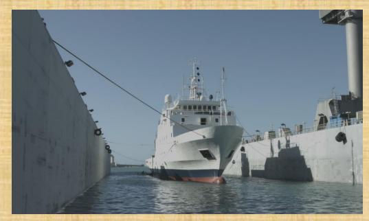
RV Urania after the welding of the new 6 meters section.
